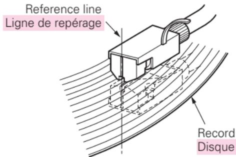
Fig. 1 Vertical View of Cartridge
