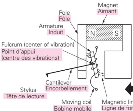
Fig. 5 Functional Diagram of Power Generation
