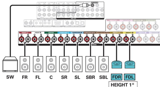
\* The surround Dolby or back Dolby speakers can be connected instead of the front Dolby speakers. In this case, set the Dolby Atmos Enabled speakers to be connected under "Height" - "Layout" in the menu. (☞ p. 233)
