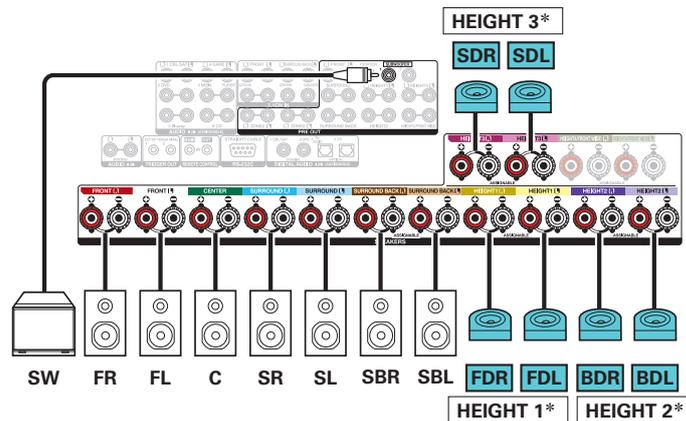
\* You can change the combination of the HEIGHT1, HEIGHT2 and HEIGHT3 channels in the settings. (📖 p. 69)
