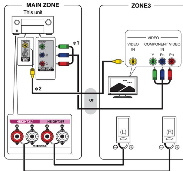
\*1 Set “ZONE2” or “ZONE3” for “Analog Video Out” - “Component” in the menu to enable use of the MAIN ZONE component video output terminal for ZONE2 or ZONE3. (🔗 p. 208)
