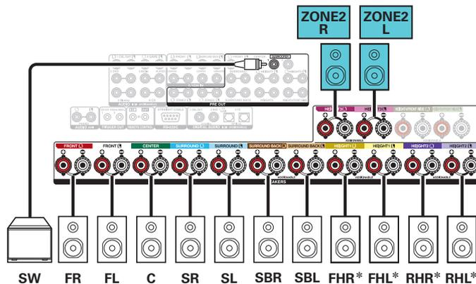
\* The height speakers, ceiling speakers and Dolby Atmos Enabled speakers can be connected to the HEIGHT1 and HEIGHT2 speaker terminals. Set the speaker to be connected from "Height" in the menu. (p. 231)
