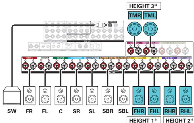
\* You can change the combination of the HEIGHT1, HEIGHT2 and HEIGHT3 channels in the settings. (👉 p. 69)
