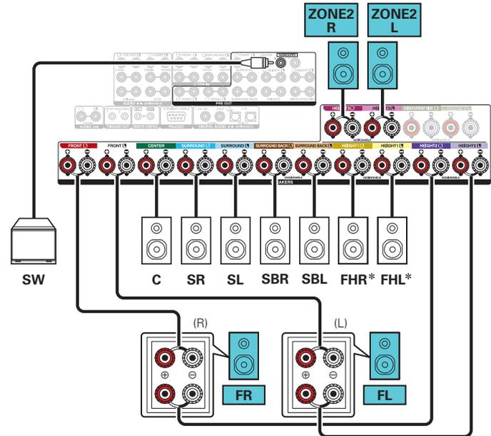
\* The height speakers, ceiling speakers and Dolby Atmos Enabled speakers can be connected to the HEIGHT1 and HEIGHT2 speaker terminals. Set the speaker to be connected from "Height" in the menu. (p. 231)
