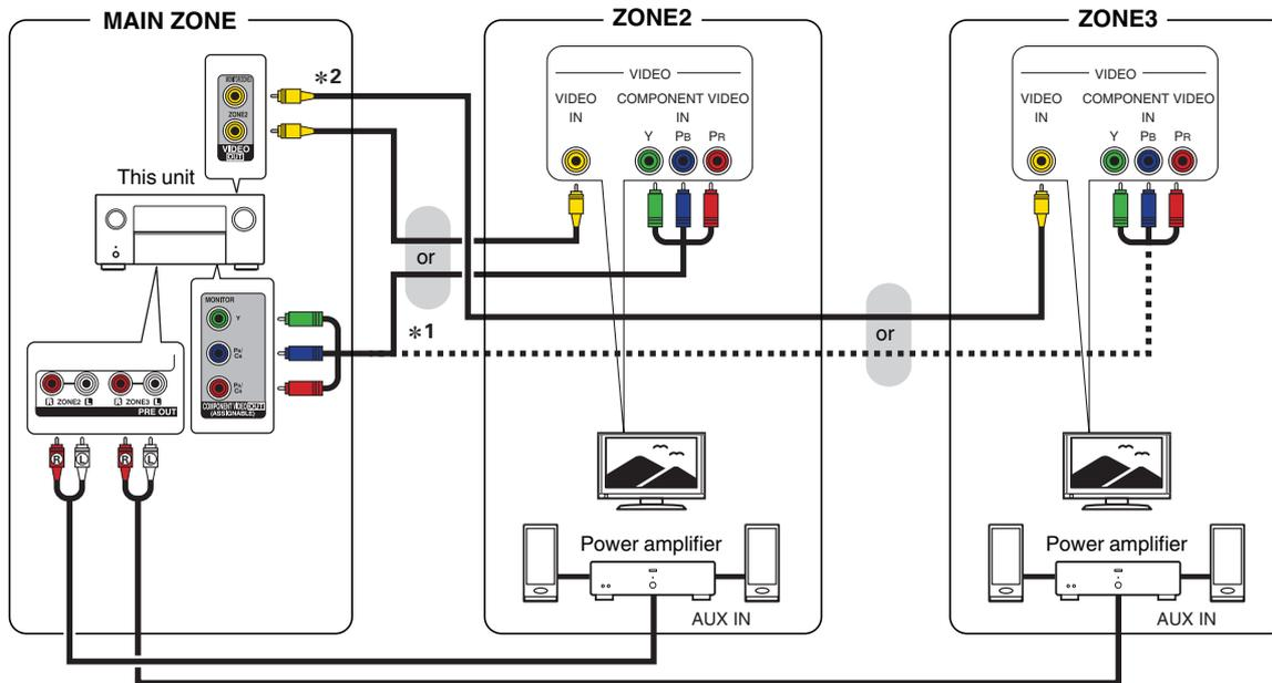
\*1 Set "ZONE2" or "ZONE3" for "Analog Video Out" - "Component" in the menu to enable use of the MAIN ZONE component video output terminal for ZONE2 or ZONE3. (☞ p. 208)
