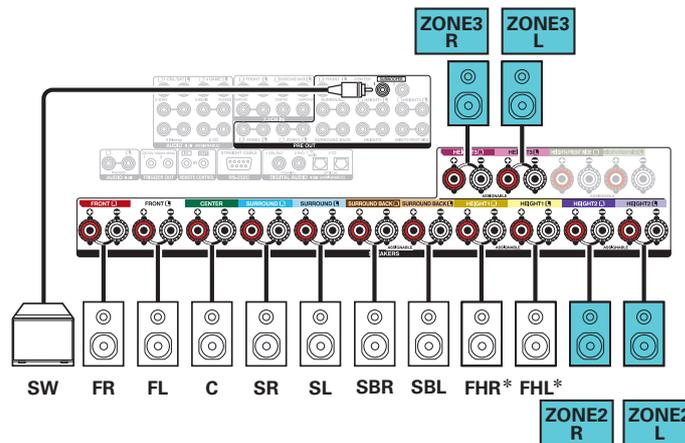
\* The height speakers, ceiling speakers and Dolby Atmos Enabled speakers can be connected to the HEIGHT1 and HEIGHT2 speaker terminals. Set the speaker to be connected from "Height" in the menu. (p. 231)
