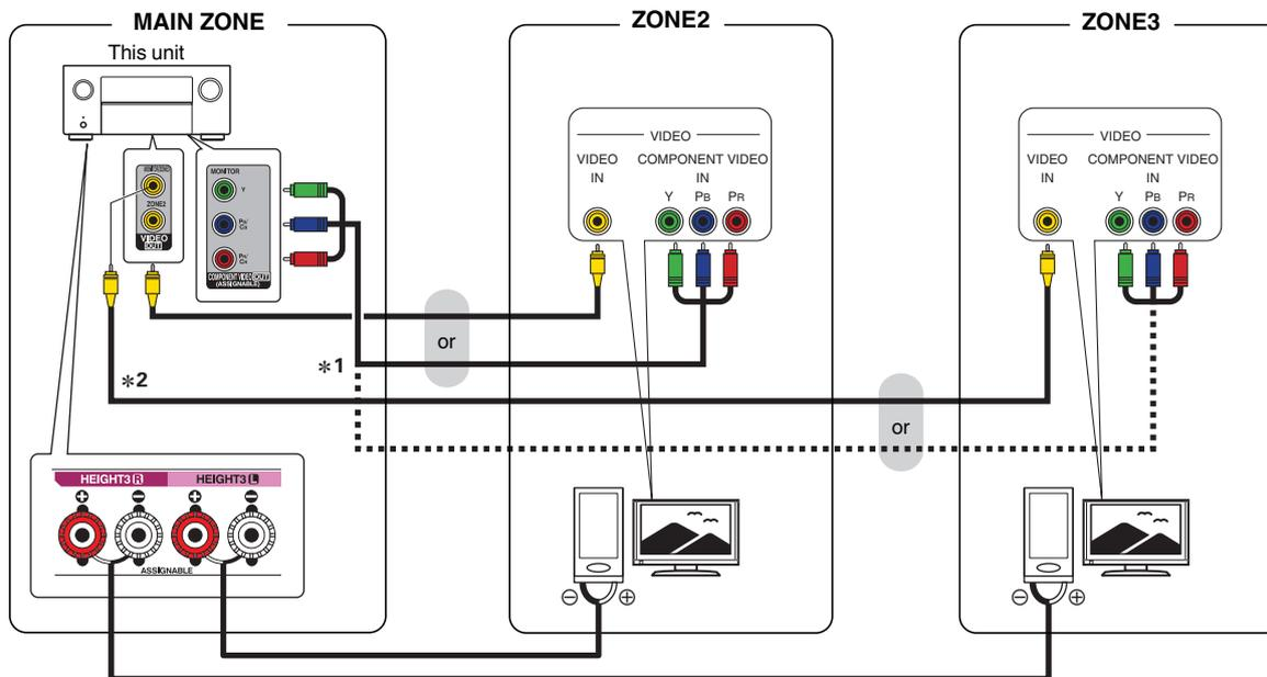
\*1 Set "ZONE2" or "ZONE3" for "Analog Video Out" - "Component" in the menu to enable use of the MAIN ZONE component video output terminal for ZONE2 or ZONE3. (☞ p. 208)
