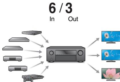
For connection to a broad range of digital sources, this unit features 6 HDMI inputs, that lets you quickly and conveniently connect a camcorder, game console or other HDMI-equipped device. There are dual HDMI outputs for the main room, and a third HDMI output for ZONE2.
