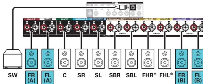
\* The height speakers, ceiling speakers and Dolby Atmos Enabled speakers can be connected to the HEIGHT1 speaker terminals. Set the speaker to be connected from “Height” - “Layout” in the menu. (☞ p. 202)
