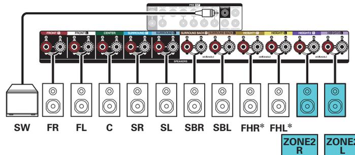
\* The height speakers, ceiling speakers and Dolby Atmos Enabled speakers can be connected to the HEIGHT1 speaker terminals. Set the speaker to be connected from "Height" - "Layout" in the menu. (☞ p. 202)
